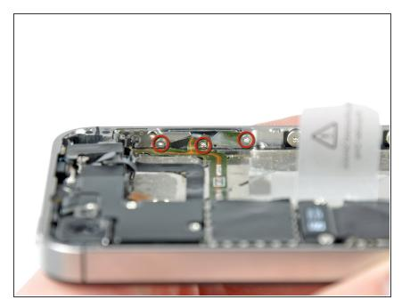
Remove the three 1.5 mm Phillips screws securing the volume button bracket to the outer case.
