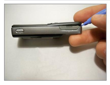
• Gently pry open the front casing by working an opening tool along the entire seam.
