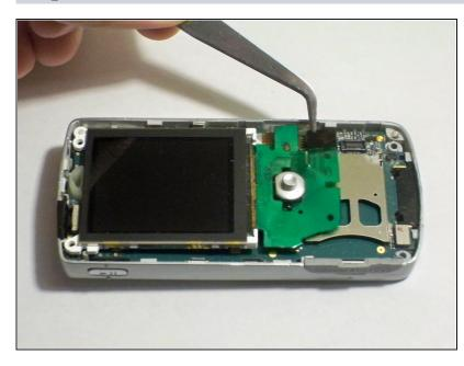
Using tweezers, insert the new joystick in place of the previous joystick.
