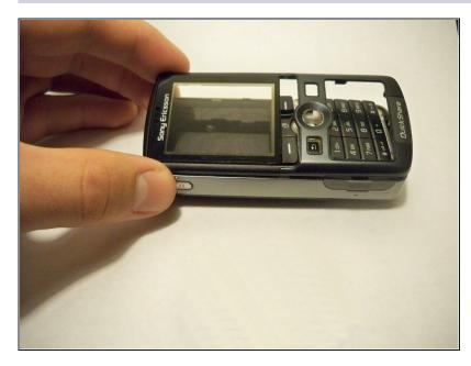
Remove the front casing by gently lifting it from the phone.
