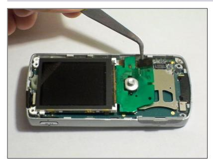
• Remove the front cover and casing to expose the joystick.
