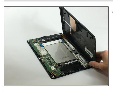
After all of the clips have been opened, the back panel should be free to remove by hand
