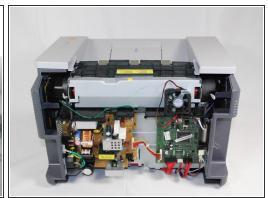
Gently lift the top panel while simultaneously pulling off the back panel.
