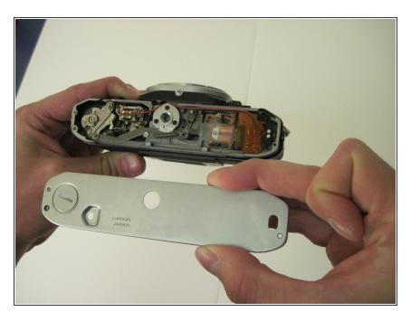
Lift and remove the bottom cover from the camera.
