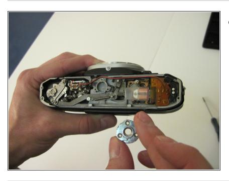
Lift and remove the tripod mount from the camera.
