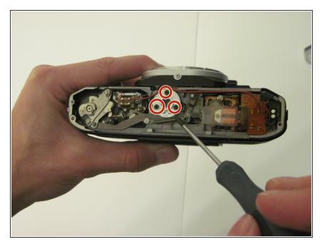
Remove the three screws securing the tripod mount using the Phillips #00 Screwdriver.
