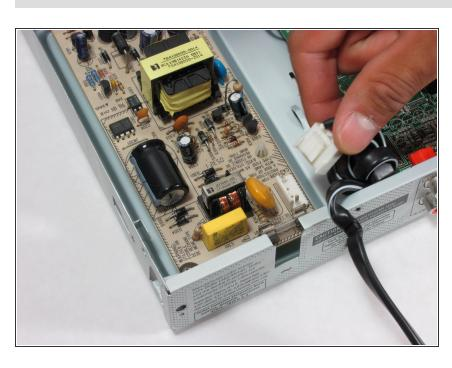
Remove the ribbon attached to the power supply by pushing the latch and gently pulling up.
