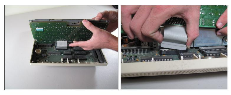
• Tilt the keyboard up while detaching the ribbon connection by pulling it straight up. You may have to wiggle the connector sideways to loosen it.
