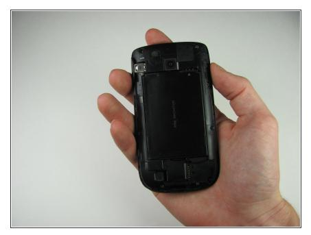
First remove the back cover of your phone to expose the battery.
