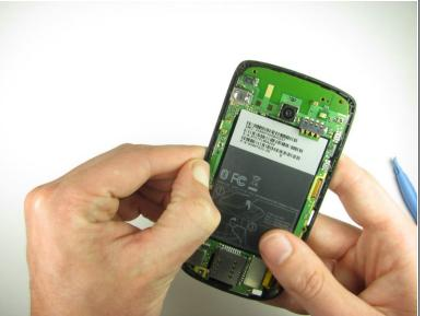
Use your finger or the plastic opening tool to unclip the board.
