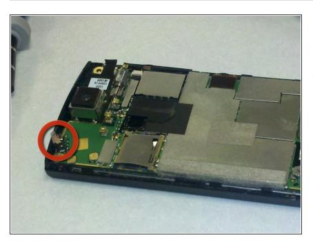
• Take the SL#2.5 screwdriver and lift up the white connector at the top right corner of the phone on the side with the circuit board
