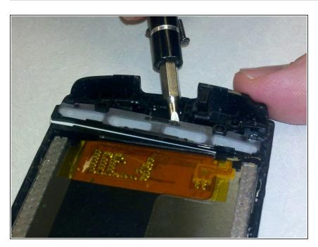
Next take the SL#2.5 screwdriver and pry the buttons off the phone and replace with the new ones
