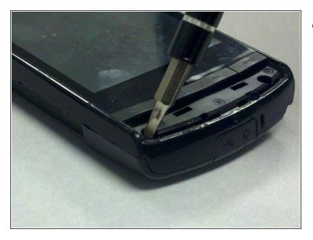
• Take a T5 screwdriver and unscrew the two screws seen here
