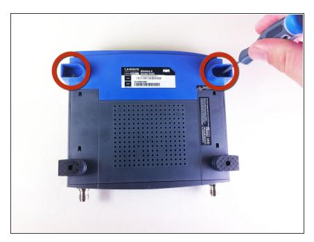
Once the feet are removed, two small screws will be visible. With a small screwdriver, unscrew them.
