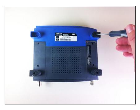
Remove the two black rubber feet of the device using the screwdriver.
