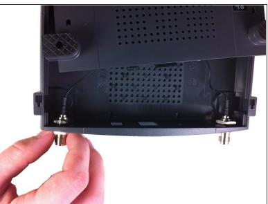
Unscrew the nut on the outer side of the back casing. Remove the nut and the washer from both antenna mounts.
