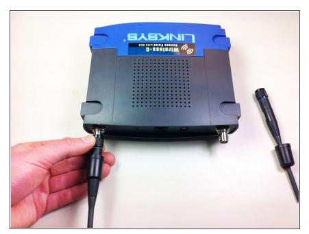
Remove the antennas from the back of the device. To do this, follow steps 1 and 2 of Installing the Antennas Guide: <u>Linksys WAP54g</u> <u>Antennas Replacement</u>
