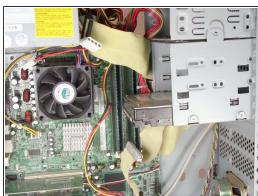
Remove the IDE data and power cables from the hard drive.
