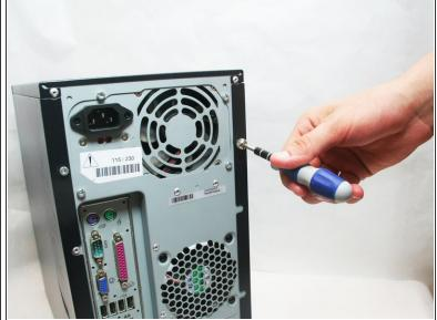
Remove the two Phillips #2 screws that secure the case door to the device.
