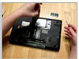
Step 3: You will then locate the screw in the top right corner, you will then pull up gently on the opening as indicated by the arrows in the pictures.
