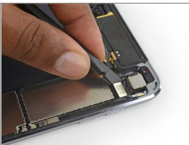
Use the flat end of a spudger to lift the rear-facing camera cable connector from its socket on the logic board.
