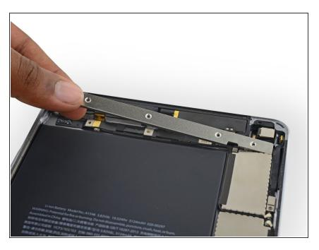
Remove the upper component cable bracket.
