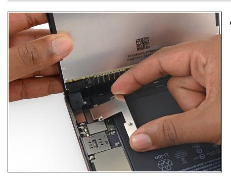
Remove the battery/display cable bracket.
