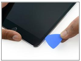
Continue sliding the opening pick down the right edge of the iPad, reheating the edge using an iOpener if necessary.
