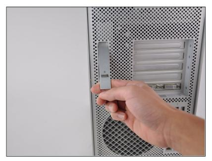
Lift the lever to unlock the case.
