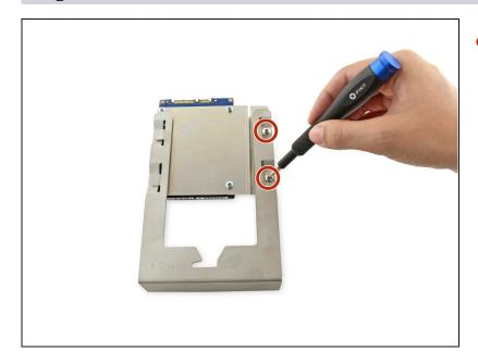
Tighten the two 7.8mm PH0 screws on the right side of the bracket.
