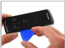
Repeat the previous step on the other side of the remote, working from the InFocus label towards the buttons until the entire cover is loose.
