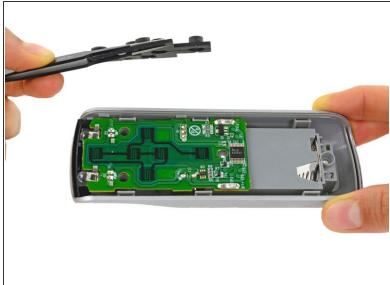
Lift the button pad up and out of the remote.
