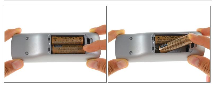
Use your finger to lift the two AA batteries up and out of the remote.
