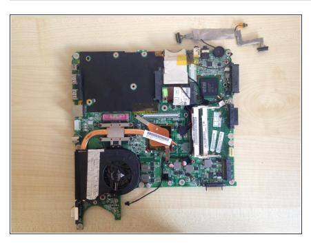
Now is an excellent time to clean the fan and the cooling vanes through which it blows air. If necessary you can use a pin to dislodge dust stuck to the heat exchanger vanes, then a vacuum cleaner crevice tool to suck it out.
