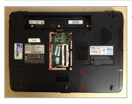
Undo two captive screws in the 2nd hard disk bay cover and remove the cover.
