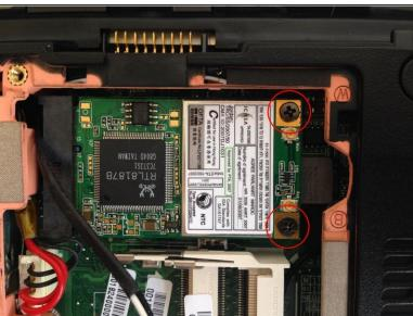
Optionally, lift the two aerial connectors off the WiFi card, remove 2 screws, and remove the WiFi card.
