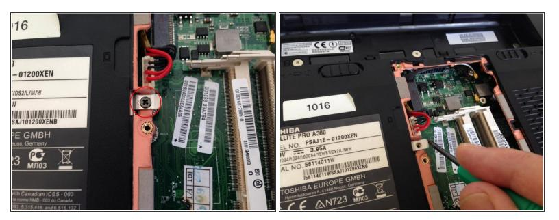
Remove the screw which retains the CD/DVD drive, and remove the drive by pushing on the tab that the screw retained.
