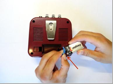
Remove the battery cover and take the battery out.
