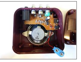
Remove the back cover by carefully pushing the battery connector through the hole in the cover.
