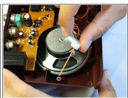
• With the phillips #0 screwdriver, unscrew the two white plastic clips that hold the speaker in place.
