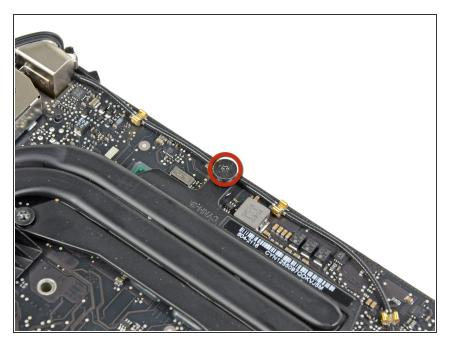
Remove the single 5 mm T6 Torx standoff from the heat sink near the edge of the logic board.
