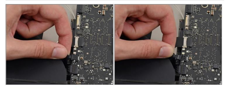
• Gently pull the fan cable connector straight out of its socket on the logic board.
