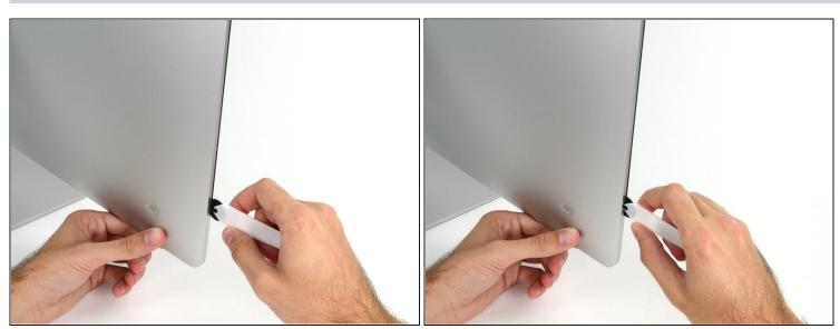
• Starting on the left of the display, near the power button, insert the iMac Opening Tool into the gap between the glass panel and the rear enclosure.
