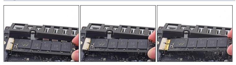
• Slightly lift the rightmost side of the SSD and firmly slide it straight out of its socket on the logic board.
