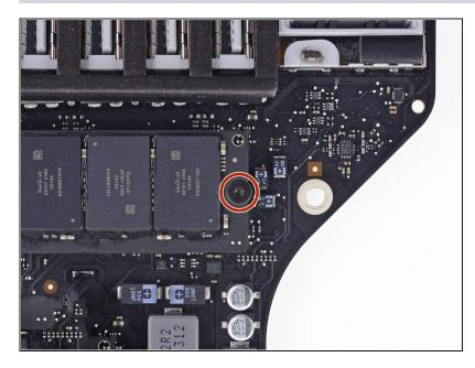
• Remove the T8 Torx screw securing the SSD to the logic board.
