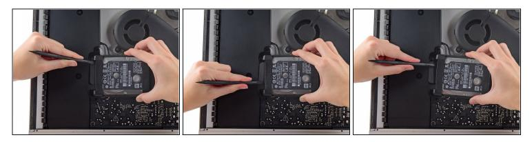
• Use a spudger to disconnect the single SATA power and data combo cable.
