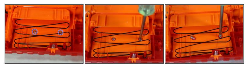
Locate the screws behind the dart pusher mechanism. Carefully remove each screw.
