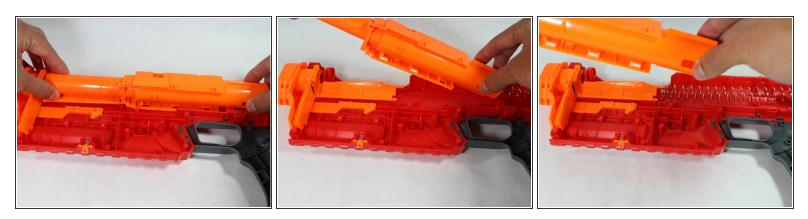
Lift the left side of the plunger tube from its peg and the rest will slide off the spring peg.
