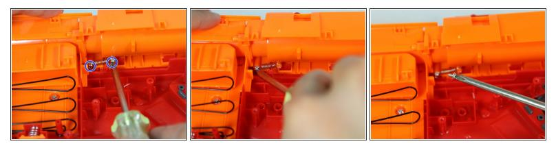
Locate the screws on the return spring. Using a counterclockwise rotation, remove both of the screws.
