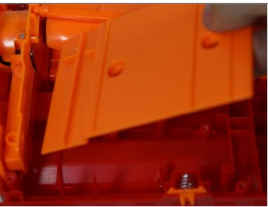
Lift up on the magazine plate in order to remove it.
