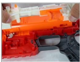
Remove the screws from the trigger mechanism and lift it upward
