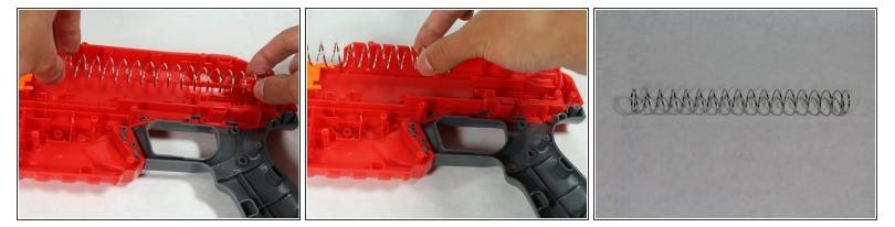
Slide the spring off its peg. If the spring is damaged, replace it.
