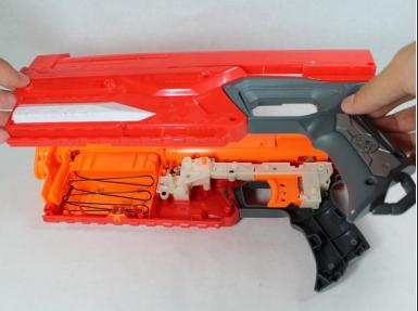
Lift up on the top half of the shell with deliberate force. This should reveal the internals.
