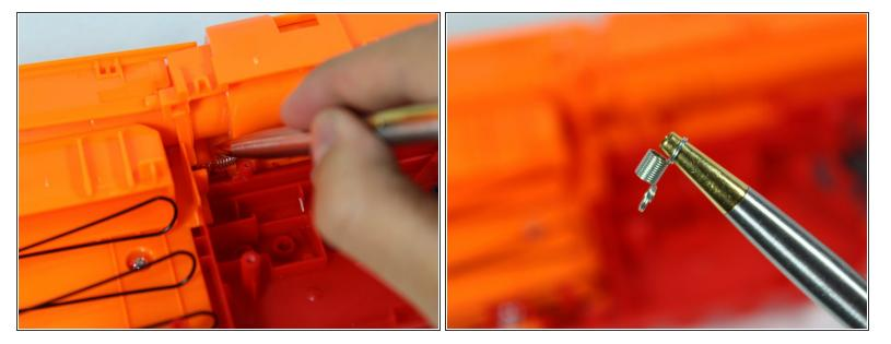
Using a small tool, carefully remove the spring from its pegs.
