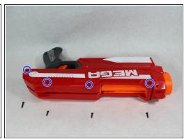
Start by removing the (4) exterior Phillips screws from the shell of the gun with a #1 Phillips Screwdriver.
