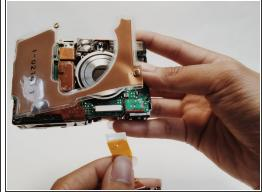
Remove the highlighted screws to remove the copper facing
