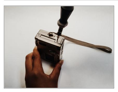
Unscrewing the small screws to take off the backing, screws are on the side and there are 4
