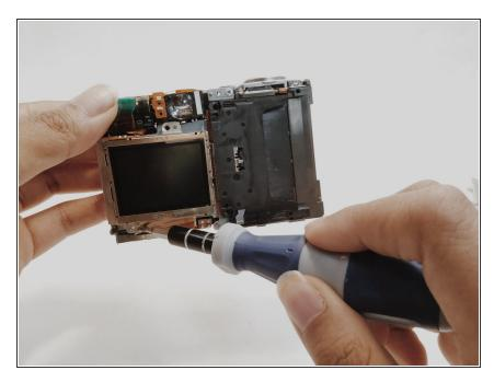
Remove the screen, also remove any screws that may get in the way, if the screen pops out it's okay, it's suppose to do that. Remove the screw at the bottom
