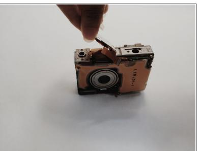
Remove screws and metal shield at the bottom of the camera
