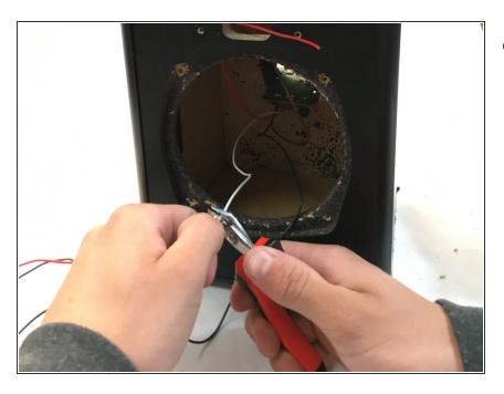
Step 4: Carefully cut the 2 wires connecting the speaker. Make sure to cut the wires about half way from the speaker.
