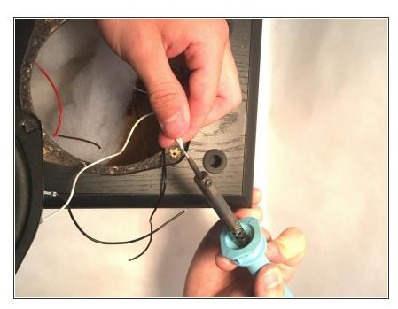
• Step 7: Solder the wires together.
