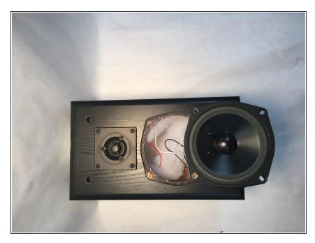
Step 3: Carefully remove the speaker from the speaker box. Be sure not to break the 2 wires connecting the speaker.
