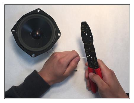
Step 6: Strip both of the wires so they are ready to be soldered together.
