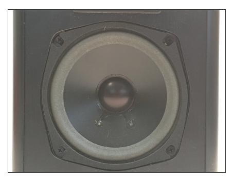
Step 8: Screw the new speaker back into the box using all 4 of the 2 cm screws.
