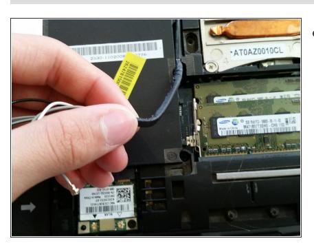
Carefully unthread the wires detached in the last step from the hooks to completely free them from the laptop.
