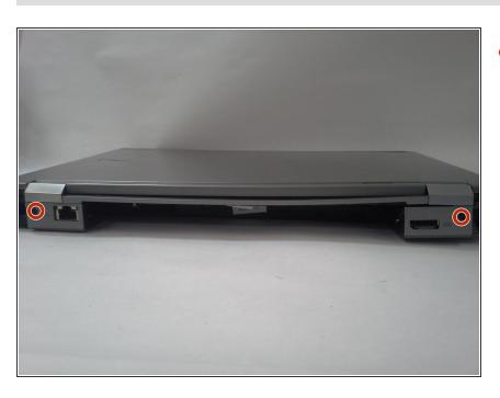
Remove the two 5 mm Phillip's screws located on the left and right side of the battery socket.
