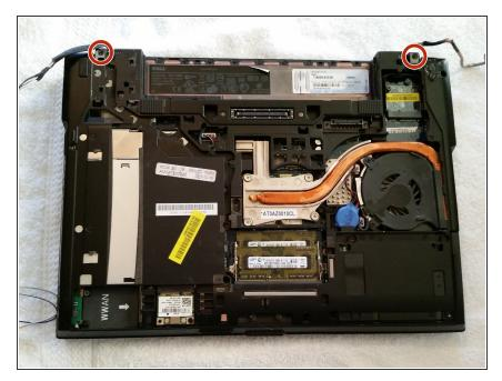
Remove the two 5mm Phillip's screws that are in the top right and left corners of the laptop.
