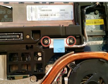
Loosen the two 5mm Phillip's screws near the top right corner that are holding the display cable onto the motherboard.
