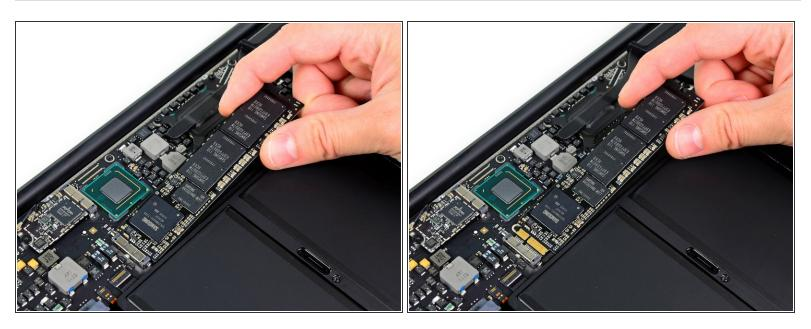
$\bigwedge$  To avoid damaging its socket, do not lift the end of the SSD excessively.
