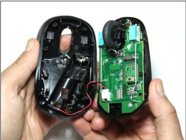
• Once the housing screws are fully removed, slowly (and carefully) separate the top and bottom halves of the housing.
