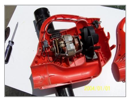
Remove rear cover. It helps to hold the plug tight to the front housing so the wires stay in place.
