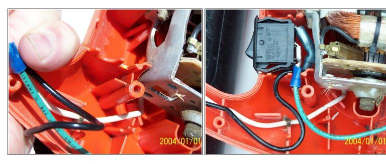
• There was not enough room for the terminal to pass by the plastic housing. I just removed a little and then routed the black wire under the switch.
