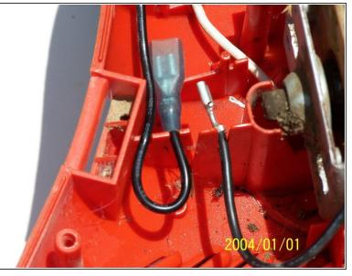
Now remove the actual electrical switch. No need to worry about the wiring, its just open and closed.
