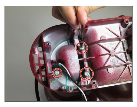
Remove the three Phillips #2 screws that connect the top portion of the mixer to the "neck" of the mixer.
