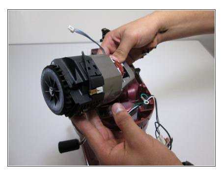
Pull upward to remove the motor.
