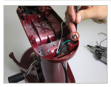
Remove the Phillips #2 screw attaching the green grounding wire to the frame of the mixer.
