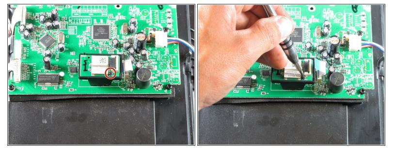
• Use a Phillips #0 screwdriver to unscrew the single 1/4 inch screw.
