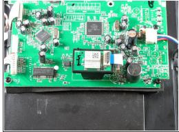
Lift the plastic tab on the ribbon cable on the bluetooth module using the spudger.
