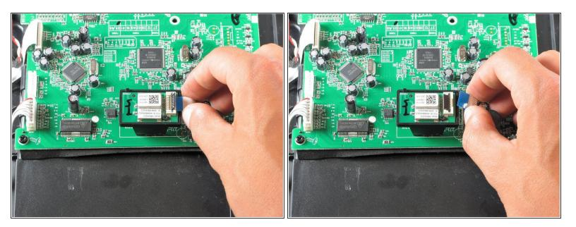
Pull the ribbon cable out to remove it.
