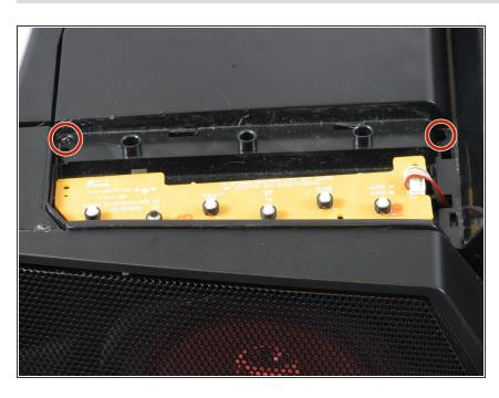
Use your Phillips #2 screwdriver to remove the two 1/2 inch screws underneath the now-removed panels.
