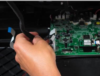
Disconnect the antenna cables.
