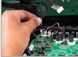
• Disconnect the remaining cables from the motherboard.
