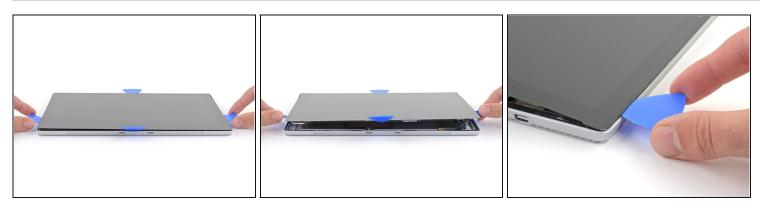
• Very slowly lift the screen assembly away from the Surface case. If you encounter any resistance, stop and check that all the adhesive is separated.
