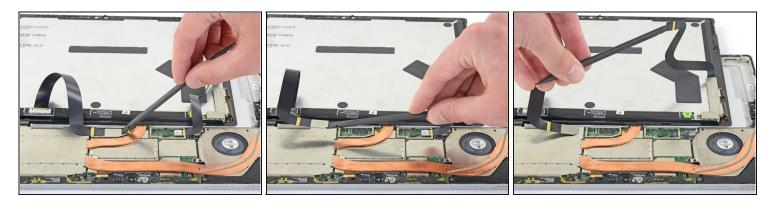
• Pry up with the flat end of a spudger to disconnect each display cable from the motherboard.
