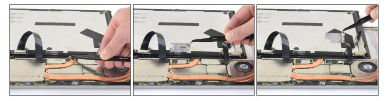
• Use your tweezers to remove the two EMI shields covering the display cable connectors.
