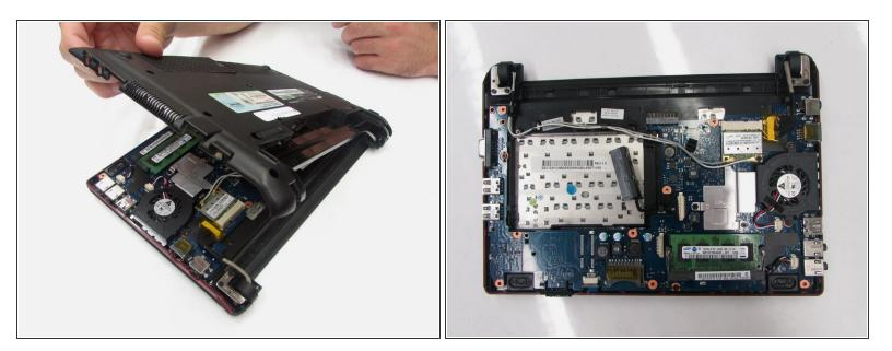
The computer should be open with the motherboard exposed and internal components exposed. You should now be able to access the Fan and RAM. There are more necessary steps to follow before accessing the screen and keyboard.
