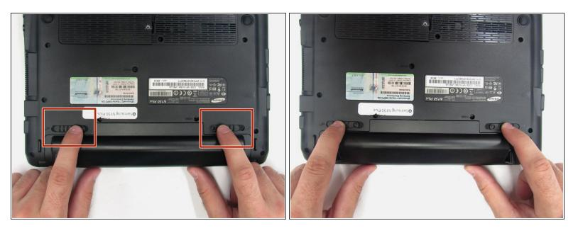
Slide the left and right switch to the "unlocked" position.
