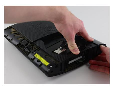
Remove the back panel by pressing down the tab on the right side of the device, and sliding the panel to the left.
