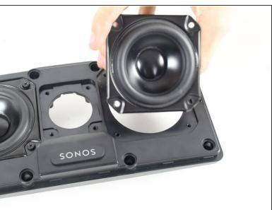
Carefully lift the speaker you need to replace out the front of the panel.
