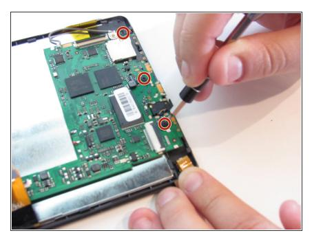
Use Phillips #000 screwdriver to remove the three 3mm screws on the motherboard.
