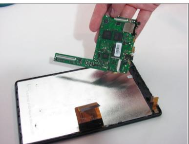
Use a spudger or plastic opening tool to lift up the motherboard.
