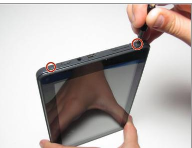
Remove the two 5mm screws from the bottom of the device using a Phillips #000 screwdriver.
