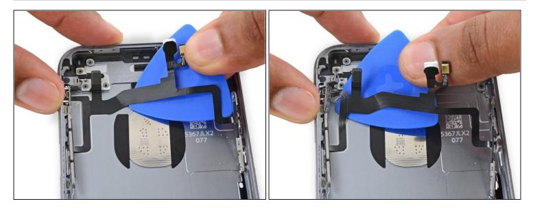
• Continue pushing the opening pick under the cable until it fully separates from the rear case.
