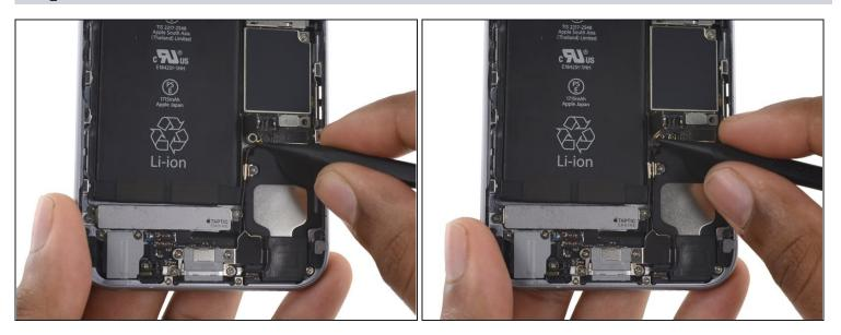
• Use the pointed tip of a spudger to disconnect the antenna cable from its socket on the lower left corner of the logic board.
