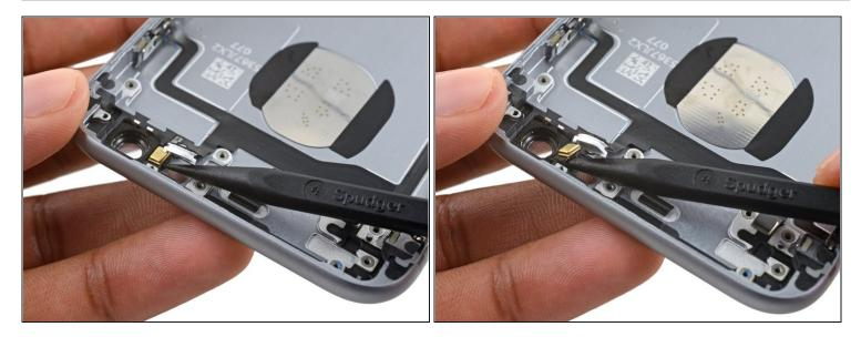
• Use the pointed tip of a spudger to gently separate the microphone from the rear case.
