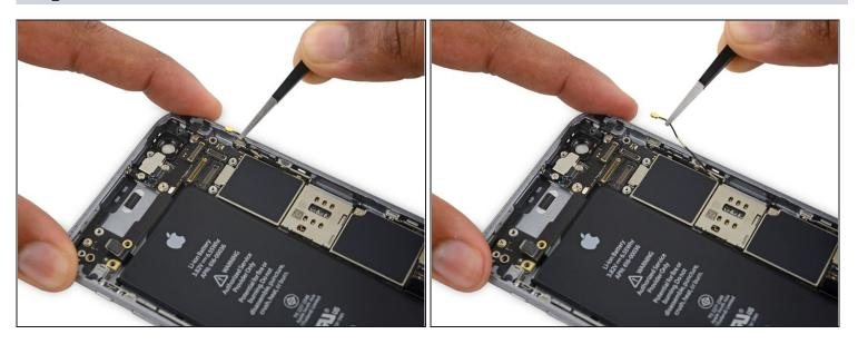
• Gently pull up on the antenna cable to de-route it from the two clips on the right side of the logic board.
