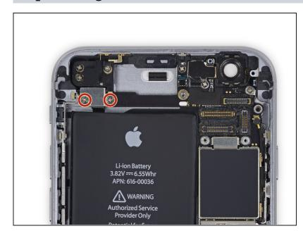
Remove the two 2.3 mm Phillips screws securing the upper component cable connector bracket.
