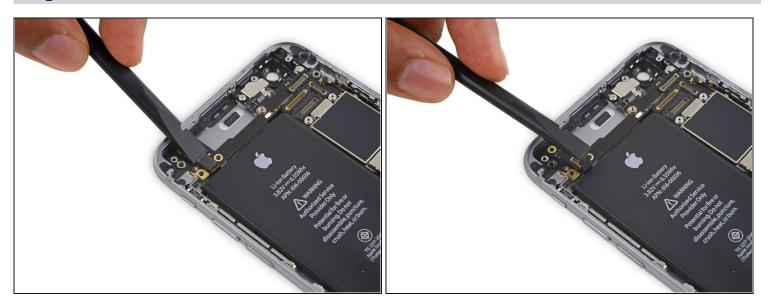
• Use the flat end of a spudger to disconnect the audio control cable from its socket on the logic board.
