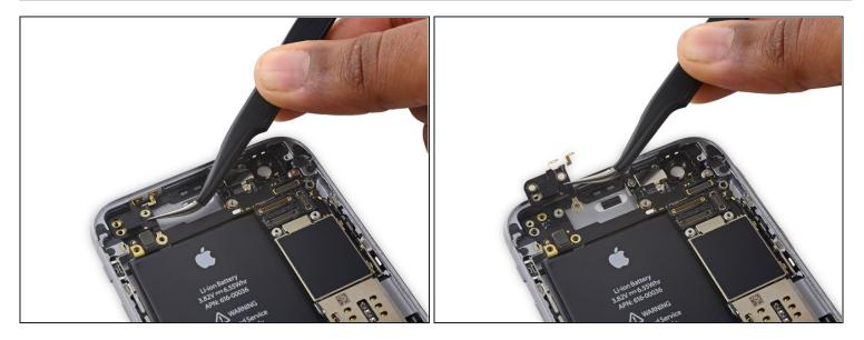
• Remove the top left Wi-Fi antenna.
