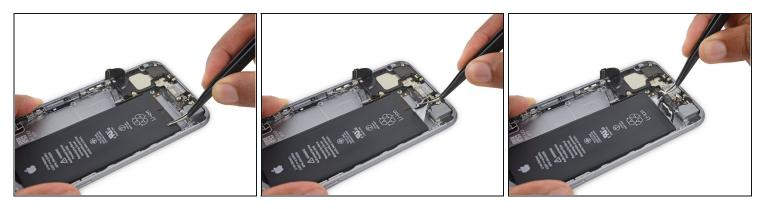
• Use <u>tweezers</u> to peel up the tips of the battery adhesive strips at the lower edge of the battery.
