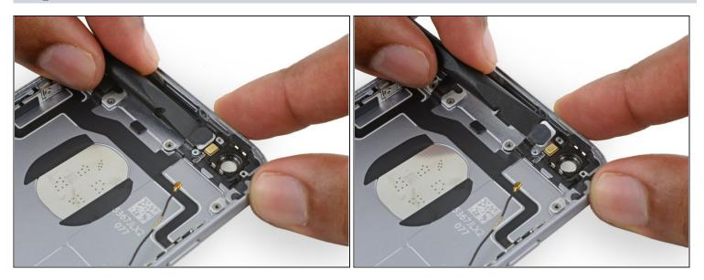
• Use the flat end of a spudger to lift the flash out of its housing in the rear case.
