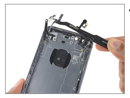
• Remove the upper component cable assembly.
