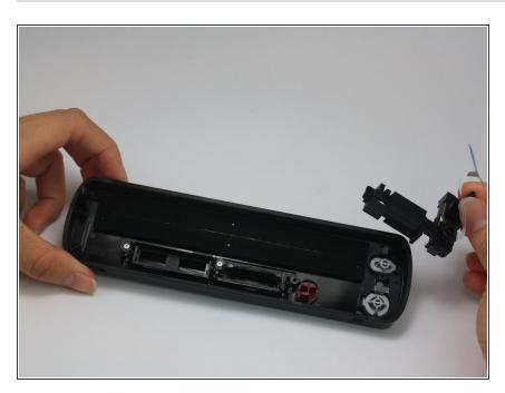
Once unscrewed, remove the black braces that hold the power button, eject button, and sync button in place.
