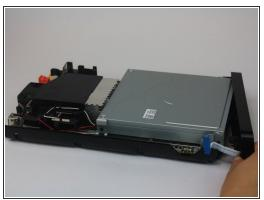
Remove the ribbon cable and separate the front plate from the main console.
