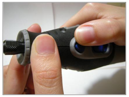
• Press and hold down on the gear lock button to lock the shaft.
