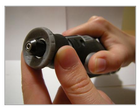
• With the lock held down, begin unscrewing the collar wrench.
