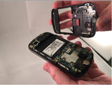
Using a spudger, separate the rear case of the phone from the front case.
