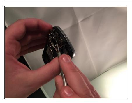
Use a spudger to peel back the green processing chip, exposing the wires underneath. Identify the thin golden band which connects the camera to the rest of the phone.
