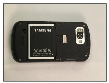
Slide the back cover off the back of the phone to reveal the battery.
