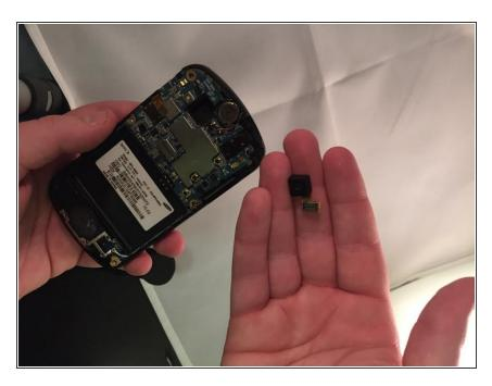
Using the spudger, separate the golden band from its resting dock. It should come apart fairly easily, like undoing a bit of velcro. Once separated, the camera should slide out.
