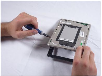
Using a spudger or plastic opening tool, carefully pry the screen bezel away from the silver midframe. To reassemble your device, follow these instructions in reverse order.
