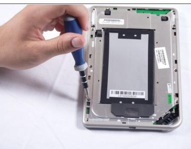
Remove the ten T5 screws from around the edges of the silver midframe.
