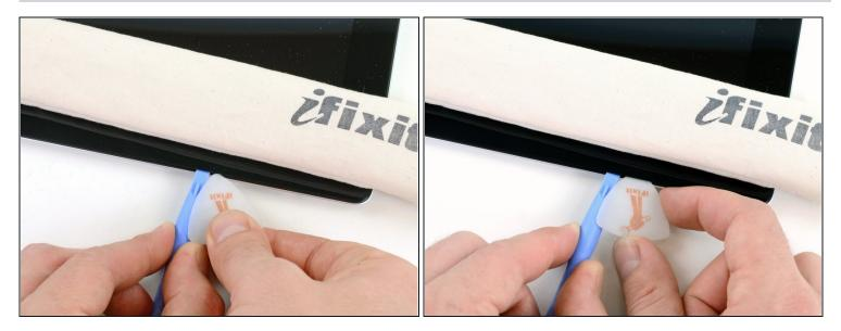
• Keeping the tip of the plastic opening tool wedged between the front glass and plastic bezel, slide a plastic opening pick in the gap, right next to the plastic opening tool.
