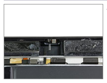
• Remove the remaining foam tape covering the microphone ribbon cable.
