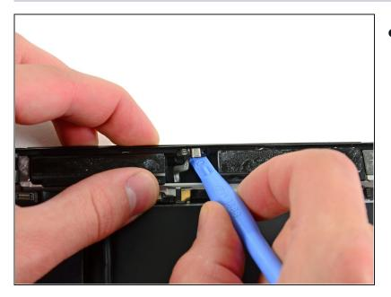
• Carefully peel the microphone off the top edge of the rear panel.
