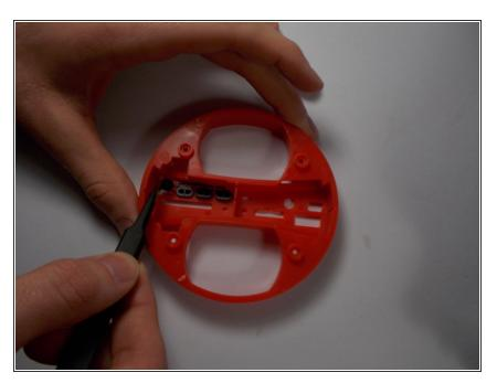
Push the set of buttons inward from the outside of the red plate and peel off from the inside.
