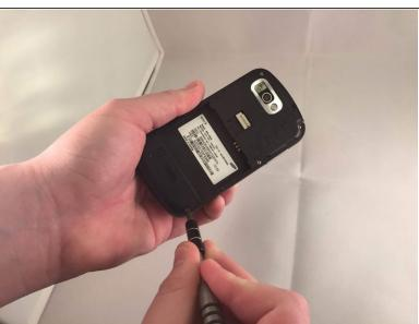
Identify and remove the 6 screws on the rear case of the phone.
