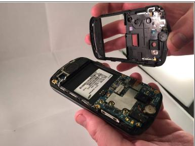
Using a spudger, separate the rear case of the phone from the front case.
