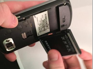
Place a finger in one or both of the indents by the bottom of the battery. Then pull out to remove the battery from the phone.
