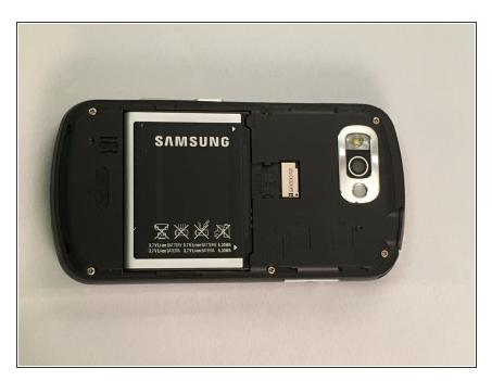
Slide the back cover off the back of the phone to reveal the battery.
