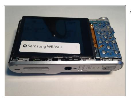
Remove the plastic casing, exposing the inner workings of the camera.
