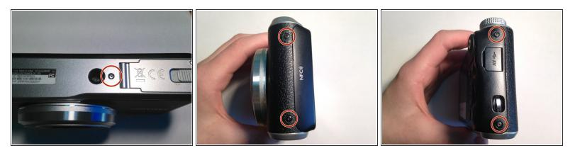
• Remove five 3.2 mm screws with a Phillips #000 Screwdriver.
