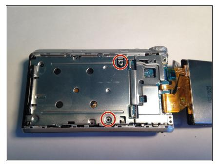
Remove two more 3.2 mm screws on the silver panel using your Phillips #000 Screwdriver.
