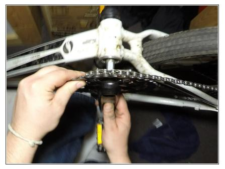
Remove the crank arm and chainrings by pulling the crank arm away from the bicycle frame.
