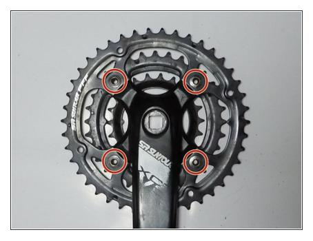
Remove the four 5 mm Hex screws that mount the crank arm to the chainrings.
