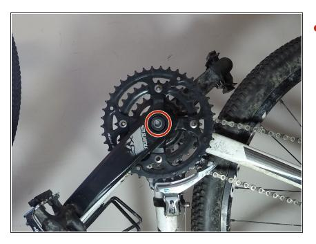
Remove the 8 mm Hex screw from the crank arm.
