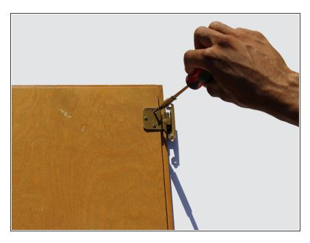
Next using a screwdriver, remove the screws attaching the hinge to the door.
