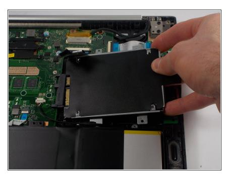
Carefully disconnect the hard drive from its port by sliding it to right.
