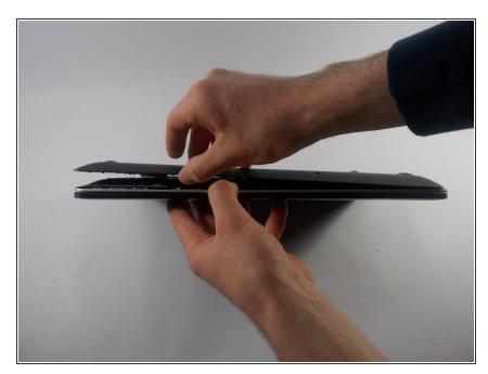
Carefully peel the panel off of the bottom of the laptop.
