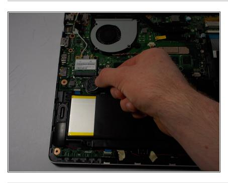
Carefully remove the CMOS battery from its port by lifting it upward.
