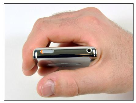
i Before opening your iPod, ensure that the hold switch is in the locked position. The slider should be all the way to the right if your iPod is facing you.
