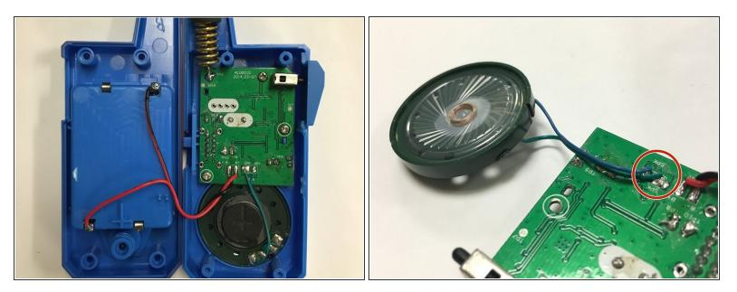
• Use a soldering device to break the connections pictured and remove the wires.
