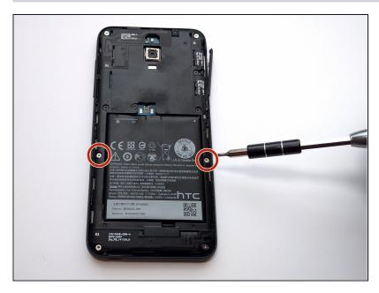
Using Phillips 000 Screwdriver, remove the two 2.5mm phillips head screws.
