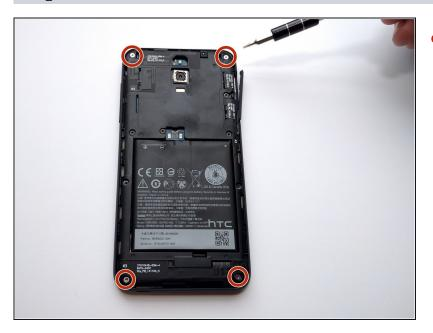
Using Torx T5 screwdriver, remove the four silver 5mm torx head screws.
