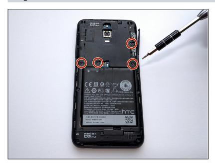
Using Torx T5 bit size, remove the four black 4mm torx screws.
