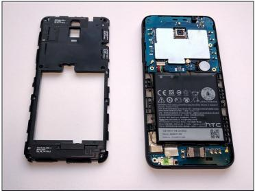
• Using plastic opening or prying tool, remove the black plastic circuit cover.
