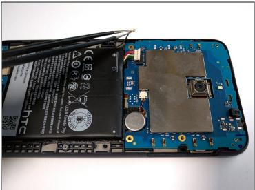
• Using <u>tweezers</u>, disconnect the antenna wire.
