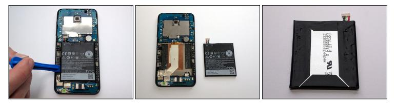
• Use the plastic opening tool - you can use a larger one, or keep using the small one - to pry out the battery.
