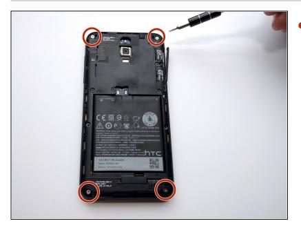
Using Torx T5 screwdriver, remove the four silver 5mm torx head screws.
