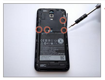
• Using Torx T5 bit size, remove the four black 4mm torx screws
