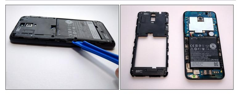
• Using plastic opening or prying tool, remove the black plastic circuit cover.
